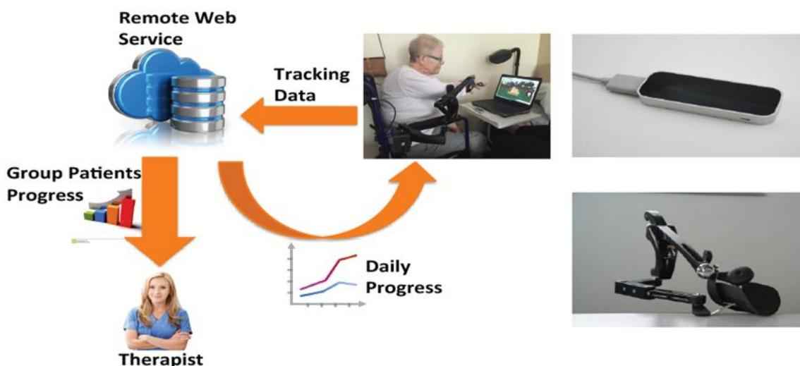
**Figure 1.** Left: RAVR-Home architecture design. Upper right: Leap Motion Controller. Lower Right: Armon Edero™ arm support.
