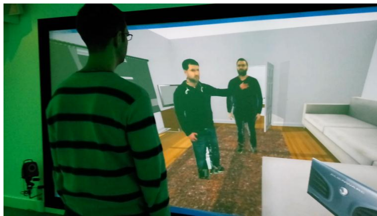
Figure 3. A mock up of a client fixating on a virtual threat and the therapist stepping in front of it. The therapist (centre) is reconstructed in real time across the telepresence link.
