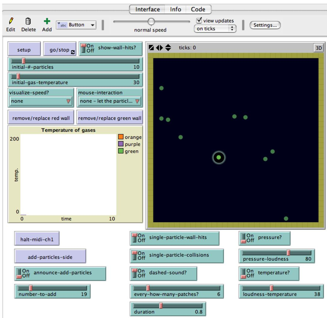
**Figure 1.** L2C sonified model of gas particles in a container. Bottom-right are variables and events that relate to a single focal particle. Bottom-middle are variables and events that relate to the group of particles.
