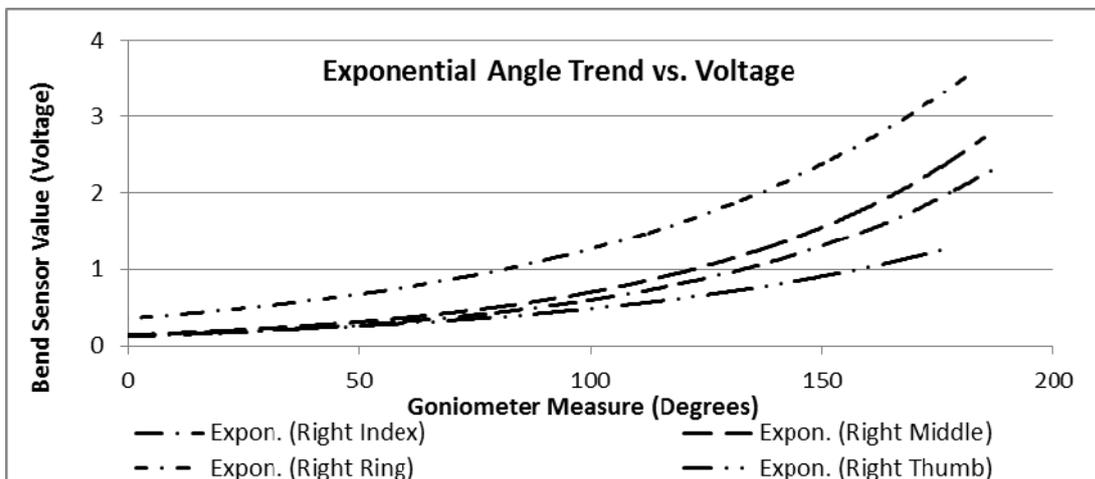
**Figure 6.** Chart of exponential angle trend vs. sensor voltage
