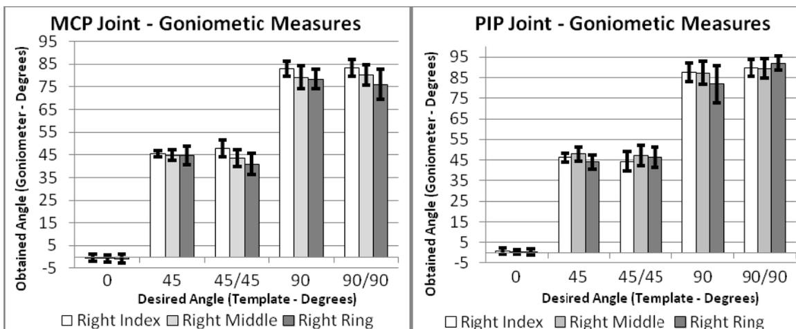
**Figure 5.** Charts of goniometric measures vs. test template
