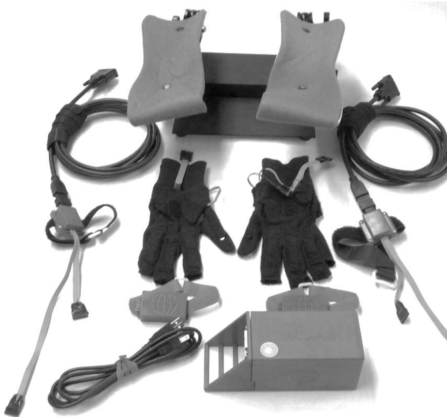
Figure 1. ATLAS bimanual glove system
