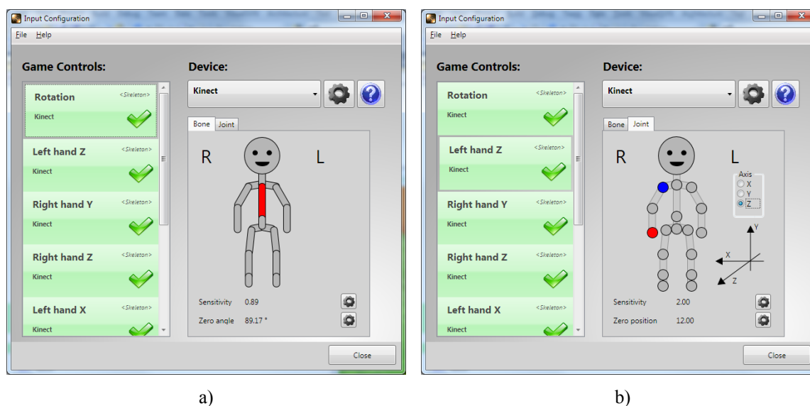
Figure 2. Configuration interface for defining input methods for games; a) input based on the rotation of segments between joints, b) input based on the relative position of joints (red – tracked joint, blue – base joint).
