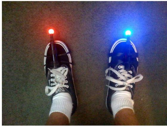
**Figure 4.** LED devices attached to right and left shoes of the user (tracked by web cameras).
