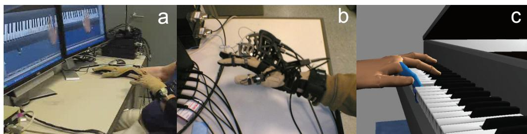
**Figure 1.** *Virtual Piano Trainer. (a) Picture of subject wearing a CyberGlove instrumented glove using the Piano Trainer Simulation; hands shown in a first person perspective. (b) CyberGrasp haptic device worn over a CyberGlove. (c) Picture of independent finger flexion as subject moves his hand to the cued key.*
