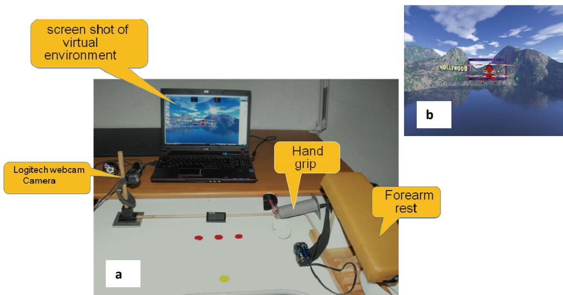
**Figure 2.** (a) Experimental setup of the adapted hand-held LED unit with hand grip, forearm rest support, web camera positioned to record motion in sagittal plane and screen shot of virtual environment. (b) enlarged screen shot of the virtual environment showing the airplane and target rectangle.
