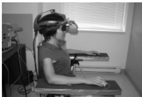
**Figure 2.** *Experimental set up. Note position of contact thermode for QST under forearm, computer mouse controls temperature changes.*
