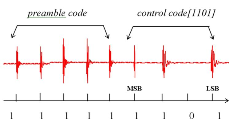
**Figure 3.** Composition of preamble and control codes.
