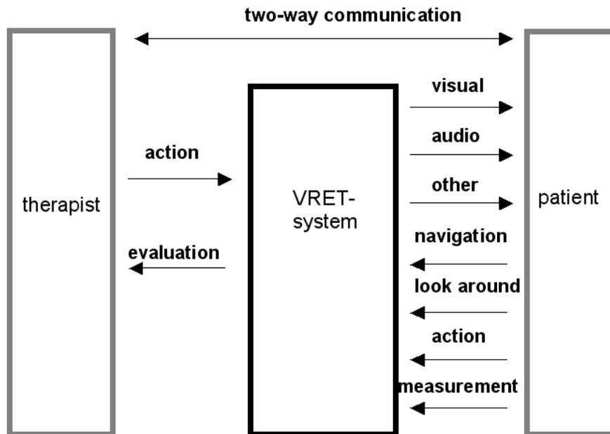
**Figure 1.** *The functional architecture of the Delft VRET system. The two-way communication of therapist and patient is direct if both are in the same room. An AV intercom connection is needed if both are not in the same room. The Delft VRET system is using two computers to be connected over the internet which supports tele-treatment.*
